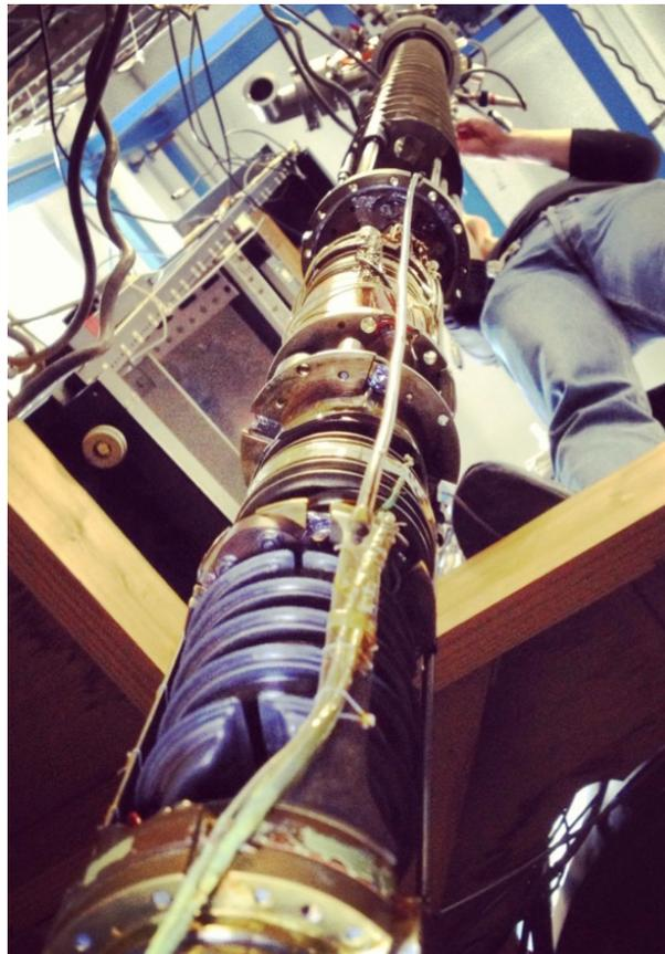
20.4 Tesla dilution refrigerator cryomagnet
